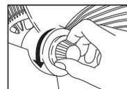
7. Tighten the blade using the spinner. Turn anti-clockwise.
