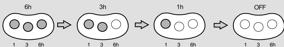
**Press the desired button to set the timer as shown above.**
